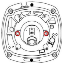
Figure 2-23 Loosen the Lens Set Screws
