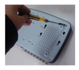
5. Fix the HDD firmly.
