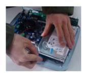
6. Connect the HDD cable and power cable.
