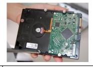
2. Fix four screws in the HDD (Turn just three rounds).
