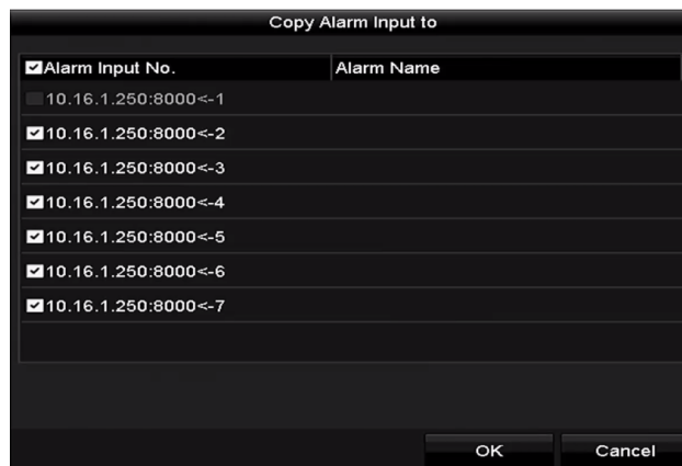
Figure 5-20 Copy Alarm Input
