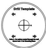
Figure 2-12 Drill Template of the Junction Box
