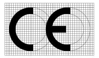
Radius of Outer Circle 100 units Radius of Inner Circle 70 units Stroke Width 30 units Length of Bar 85 units Axis to Axis 170 units Minimum Height 5.0 mm
